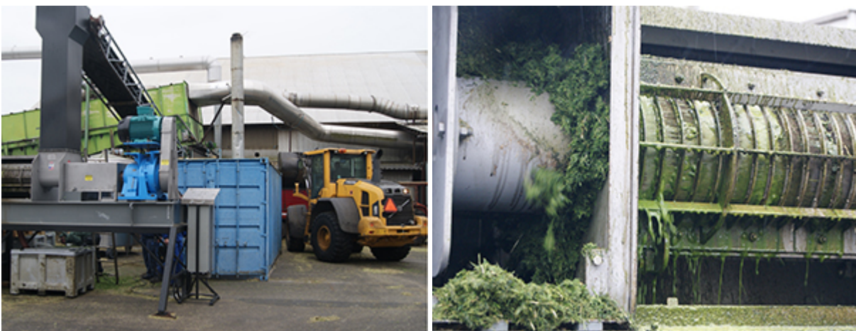
Photo 1: Full scale test plant with Vincent screw press.
